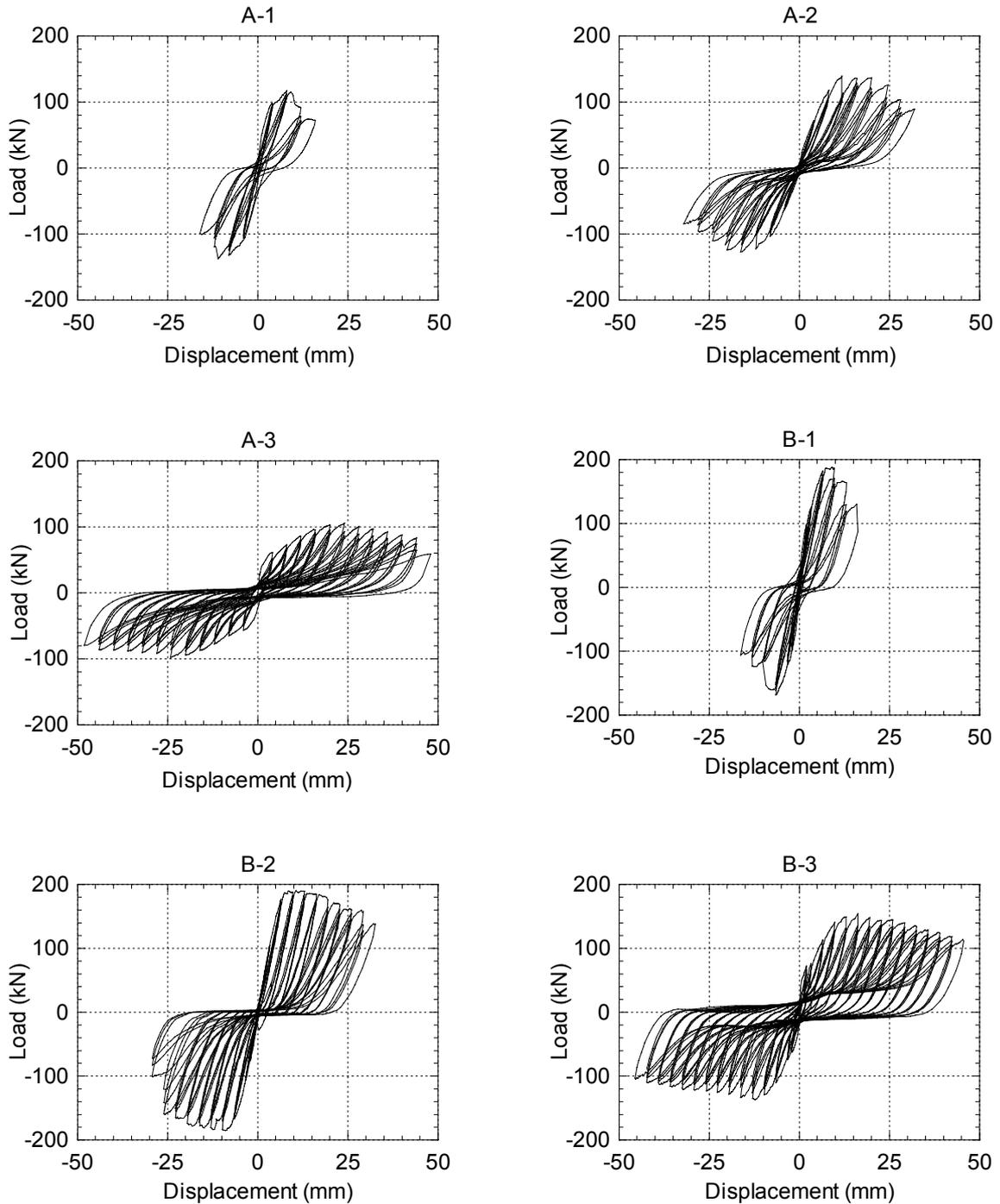
**Fig. 4-Load displacement curves of all tested specimens**
