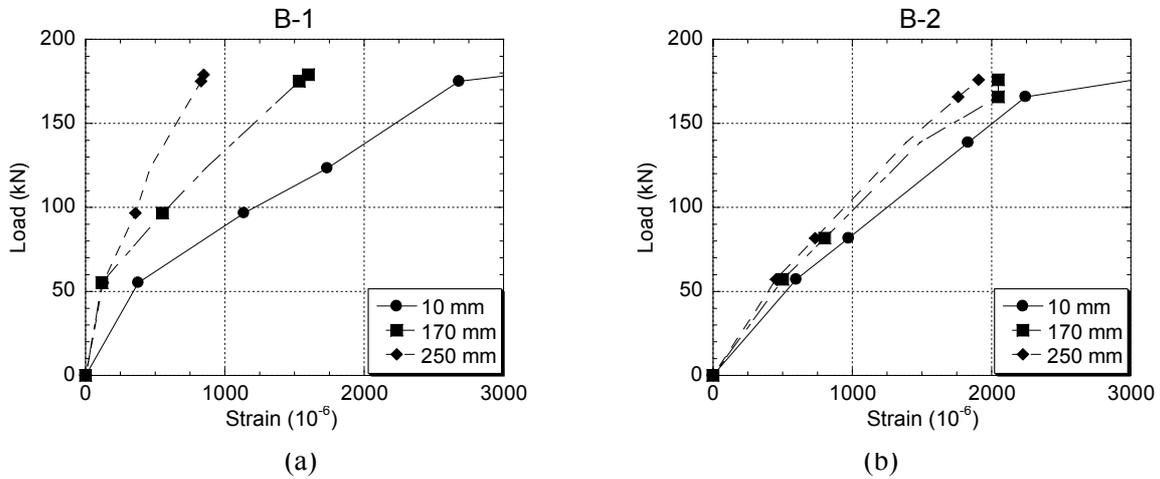
**Fig. 7- Comparison of strain at three different locations of longitudinal bars for specimen (a) B-1 and (b) B-2**
