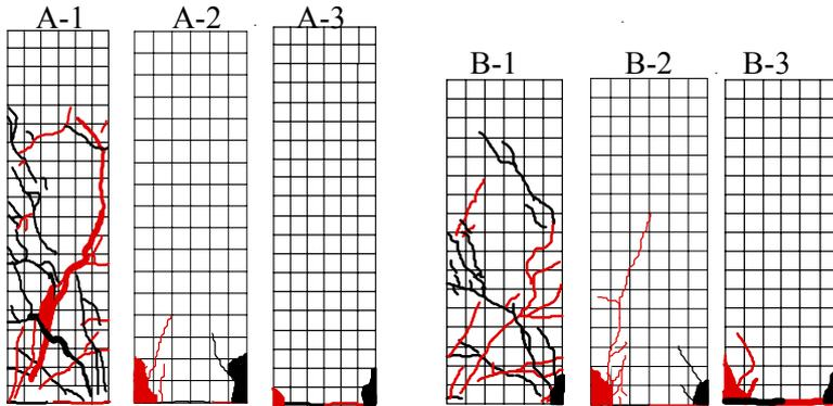
**Fig. 5-Crack pattern of specimens at failure**
