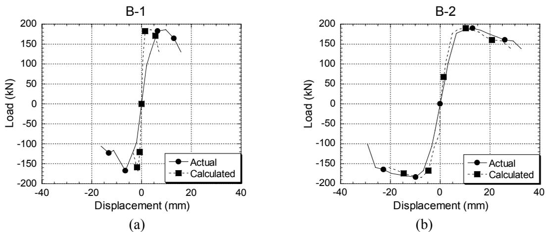
**Fig. 9-Comparison of displacement calculated by rigid body analogy with actual value**
