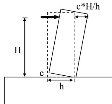
**Fig. 8-Displacement due to rigid body rotation**
