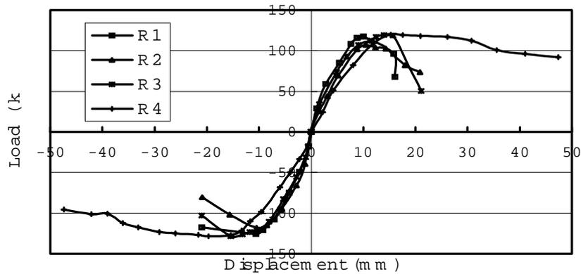
Fig.5 Load Displacement Skeleton Curves
