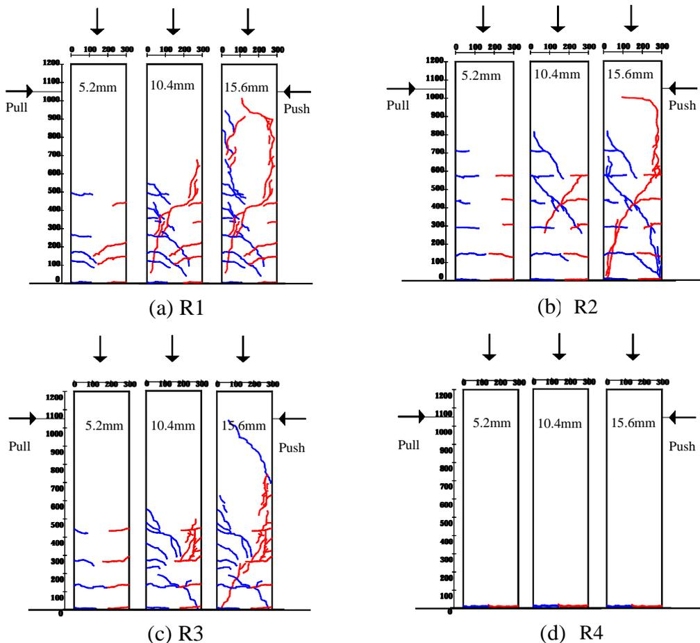
Fig.3 Crack Patterns
