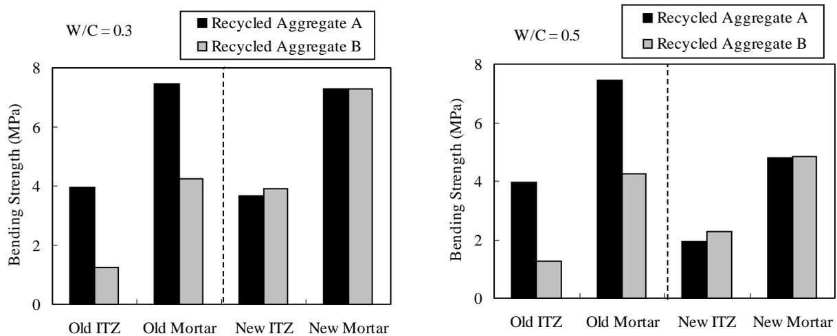
Fig. 10 Bending Strength of Micro-Regions in Recycled Aggregate Concrete
