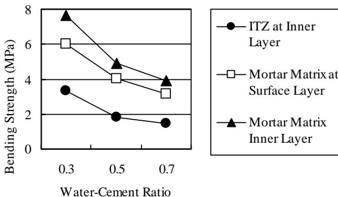
Fig. 9 Bending Strength of Micro-Regions in Concrete
