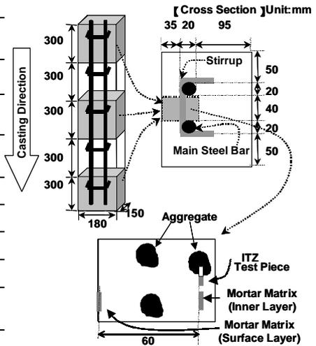
Fig. 4 Normal Concrete Specimen and Position of Test Pieces
