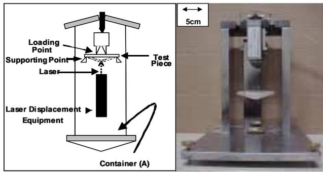
Fig.1 Micro-Bending Device
