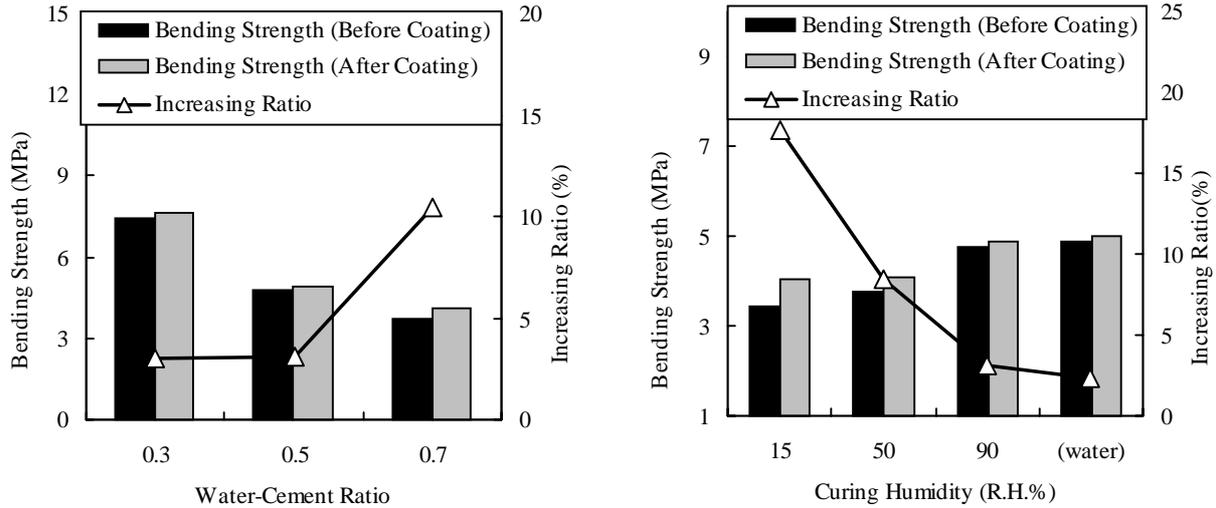
Fig.11 Bending Strength and Increasing Ratio of Bending Strength of Micro-Regions in Concrete Coated with CFRPS
