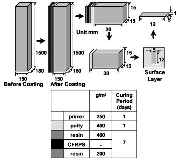
Fig.6 Concrete Coated with CFRPS Specimen and Position of Test Piece
