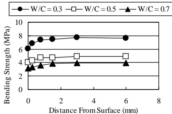
Fig.8 Bending Strength of Mortar Matrix
