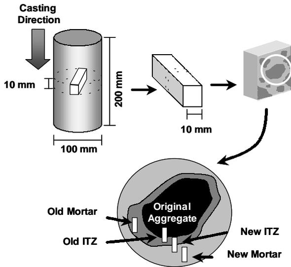
Fig.5 Recycled Aggregate Concrete Specimen and Position of Test Piece
