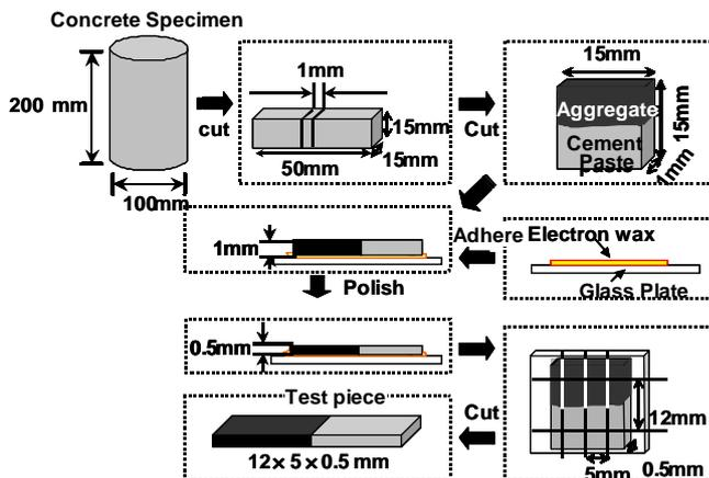
Fig. 3 Outline for Preparation of Test Piece
