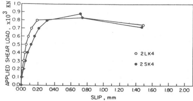
Fig. 6 Load-slip curve at the 4 MPa pre-load level (phase II)
