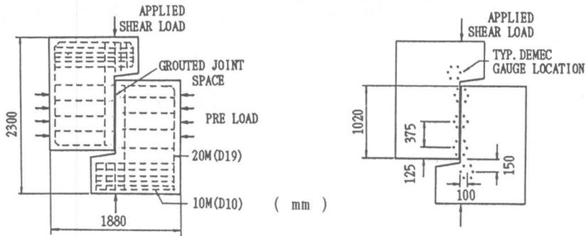
Fig. 1 Overall specimen dimensions and demec gauge location
