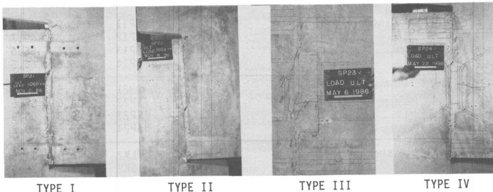
Fig. 4 Typical crack patterns (phase I)
