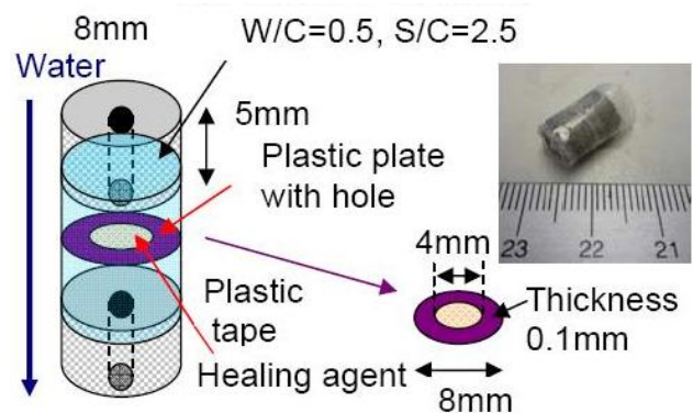
Fig.7 Schematic illustration and a picture of the water flow specimen
